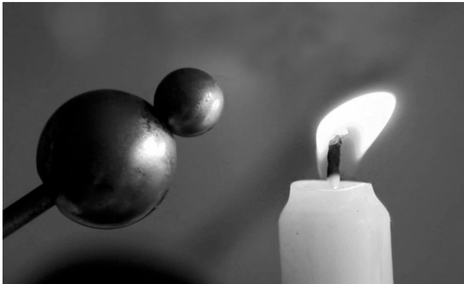
Figure 1. Deflection of a candle flame in an electric field
